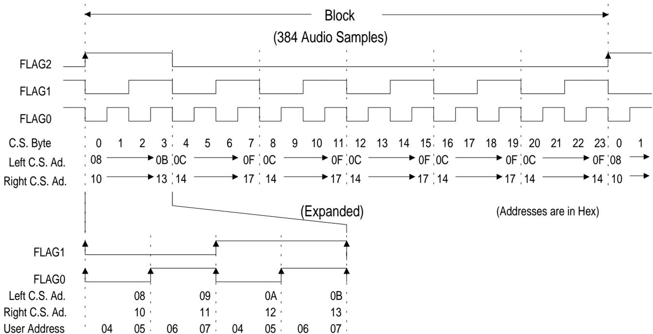
**Figure 14. CS8411 Buffer Memory Write Sequence - MODE 2**
