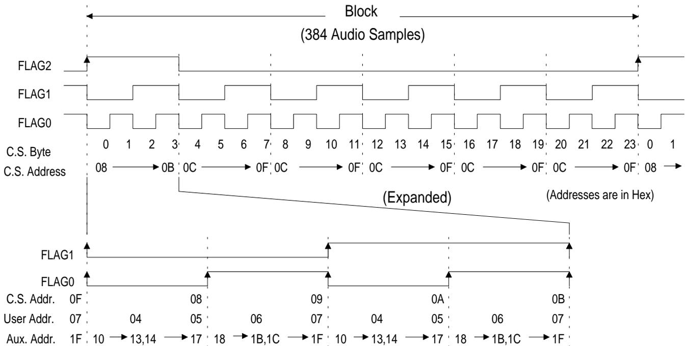
**Figure 13. CS8411 Buffer Memory Write Sequence - MODE 1**
