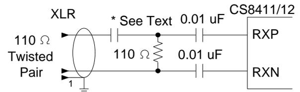
**Figure A3. Transformerless Professional Circuit**
