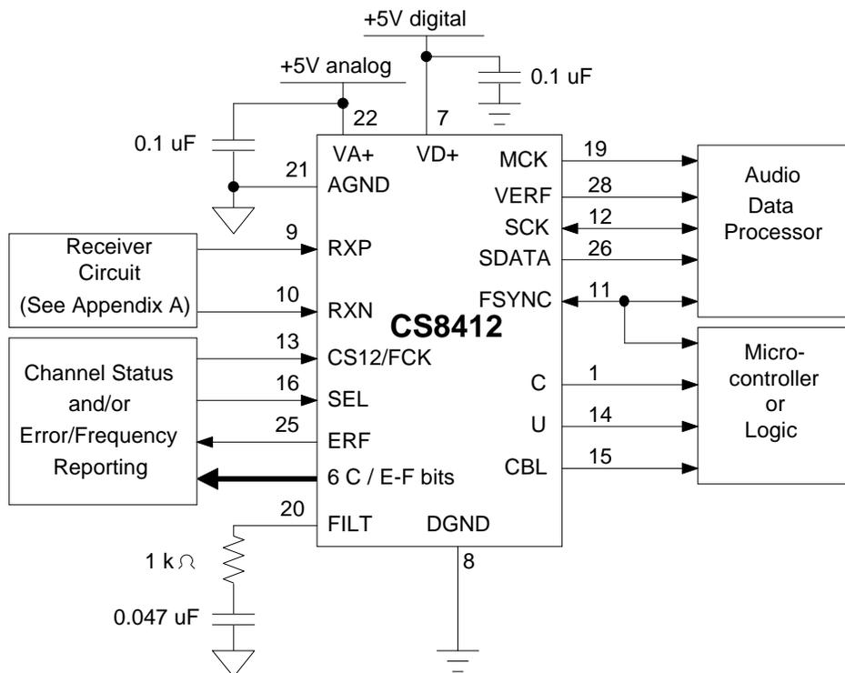
**Figure 2. CS8412 Typical Connection Diagram**
