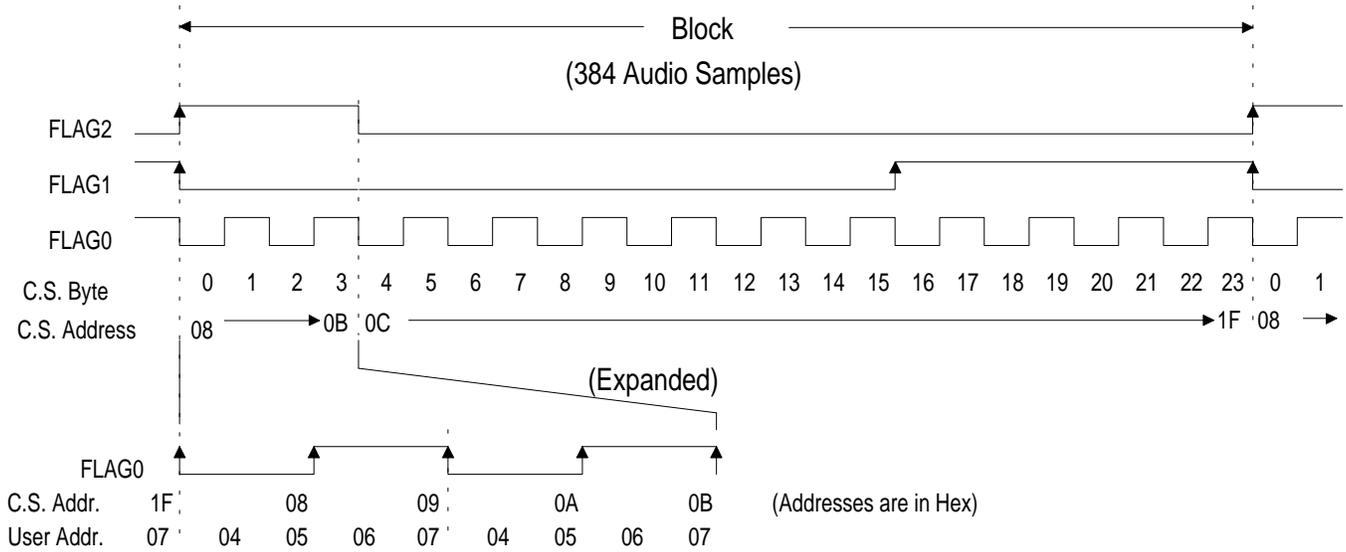
**Figure 12. CS8411 Buffer Memory Write Sequence - MODE 0**
