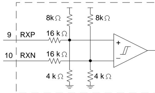
**Figure A1. RS422 Receiver Internal Circuit**
